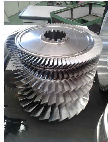
FIGURE 8. MANUFACTURED COMPRESSOR ROTOR.
