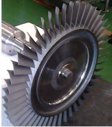
FIGURE 9. MANUFACTURED TURBINE ROTOR.
