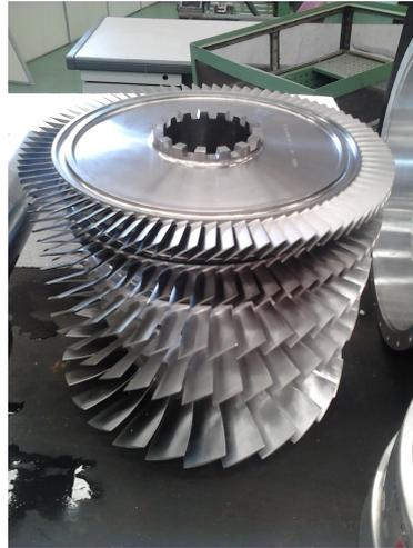
FIGURA 4.6: Rotor do compressor.
